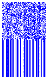
Figure 3: RBN 1d space-time pattern, n=150 , k=5 . Time proceeds from the top down. Wiring and rules were initially set at random resulting in chaotic dynamics. Midway in the space-time pattern the rules were adjusted to set canalizing inputs at 52% resulting in the rapid emergence of frozen elements, a sign of order.
