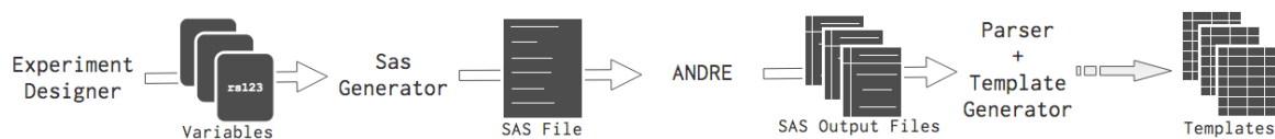
Figure 3. EAGLE project epidemiologic collection workflow. The epidemiologic collection workflow begins with the Experiment Designer, designed as a web-interface and accessed by EAGLE analysts. The analyst can easily use the Experiment Designer to create standardized SAS code based on parameters set by the analysts. The resultant ANDRE-friendly code is automatically generated. Once the code has been submitted, ANDRE will send censored output files back to the EAGLE analysts. These resultant files are first crudely parsed and stored in a database in preparation for “real-time” parsing by analysts. Finally, analysts use the “Template Generator” to create standard PAGE Results Template files for sharing data across PAGE study sites for meta-analysis.
