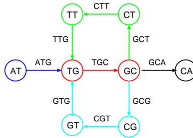
Figure 2: Example of a de Bruijn graph for sequence ATGCTTGCGTGC, with edges being all 3-mers from this sequence, and vertices being all 2-mers. Due to the repeat TGC there is another sequence ATGCGTGCCTTGCA corresponding to another Eulerian path in same de Bruijn graph (compare with Fig.1).
