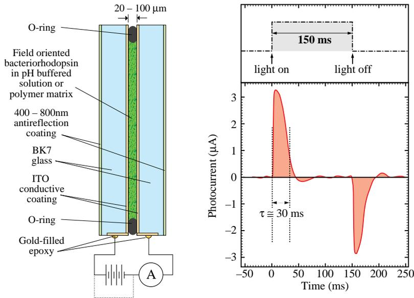
Figure 4: Bacteriorhodopsin photoelectrode and its photocurrent response
