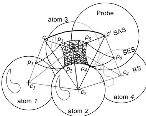
Figure 2: Probe rolling over two atoms defining an RS-edge ( $c_2, c_3$ ), an SES toroidal face ( $p_1, p_2, p_3$ ) and an SAS edge ( $c, c'$ ).
