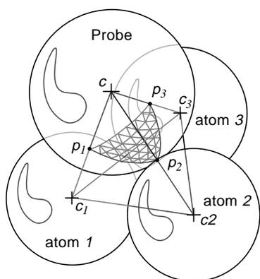
Figure 1: Probe in a fixed position defining an RS-face ( $c_1, c_2, c_3$ ), an SES spherical reentrant face ( $p_1, p_2, p_3$ ) and an SAS vertex  $c$ .
