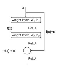
Fig. 2. A building block of Residual Network
